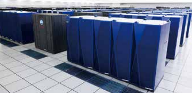
Earth Simulator is a large vector supercomputer, which is particularly suitable for simulations of the atmosphere, oceans, and other fluids.
