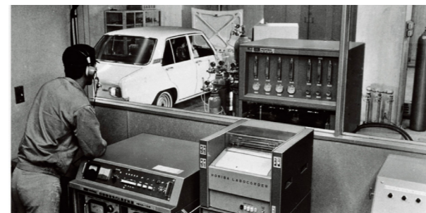
Japan's first automotive exhaust gas measurement system, MEXA
